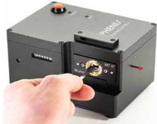
Inserting the MT ferrule
