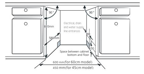
**2.** If dishwasher is in stalled at the corner of the cabinet, there should be some space when the door is opened.
