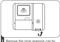
Remove the rinse reservoir cap by lifting up the handle .
