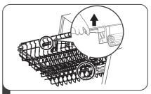
To lower the upper basket, lift the adjust handles on each side to release the basket and lower it to the lower position.
