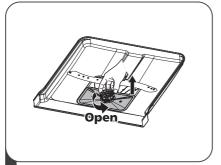
1 Hold the coarse filter and rotate it anticlockwise to unlock the filter.
