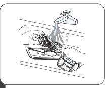
3 Larger food remnants can be cleaned by rinsing the filter under running water.
