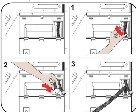
**! ATTENTION:** The hose must be connected in a manner that it cannot be displaced. If the hose comes out during water discharge, there might be flooding in your house.
