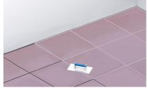
**6.** Pour ARJUNT® Universal mixed with latex resin (140 g/kg de ARJUNT®) to cover the joints.
