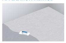
1. Spread a fine layer of ARGOCOLA® Élite 500 on one side of the floor slab.
