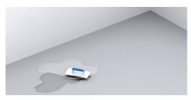
1.- Clean and prepare the substrate prior to the application of CONFORDAN, eliminating any unevenness present.
