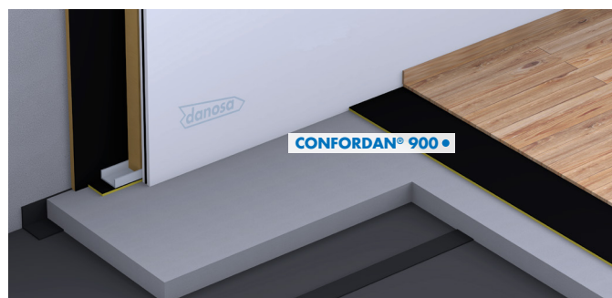
Basic floating wood floor
