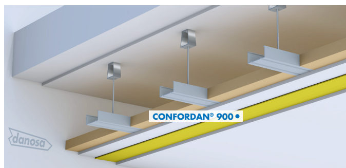
Floating roof for noisy premises, daylight hours
