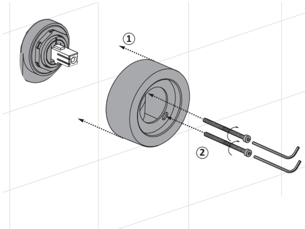
**2** Instalar el embellecedor · Install the trim · Installer la garniture
