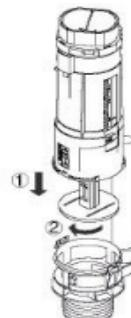
Assembly flush valve by push down and turn left.
