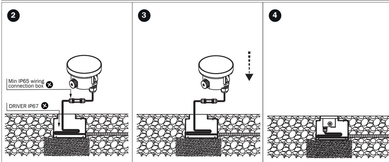
IP65 The block of connection is **not included**. The installation can need the intervention of a qualified person. The block of connection must comply EN 60998-2-1 or EN 60998-2-2. The block of connection: MAX 10A
