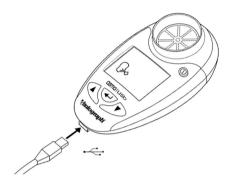
Figure 4. Attached USB cable.
