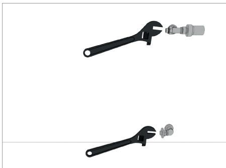
onto the lower connection of the emitter exchanger and level the equipment, marking the location of the holes provided for its fastening on the wall. Remove the exchanger by disconnecting it from the lockshield and proceed to drill holes in the facing and place the plugs and screws supplied with the equipment. Hang the exchanger from the heater and check its levelness.
