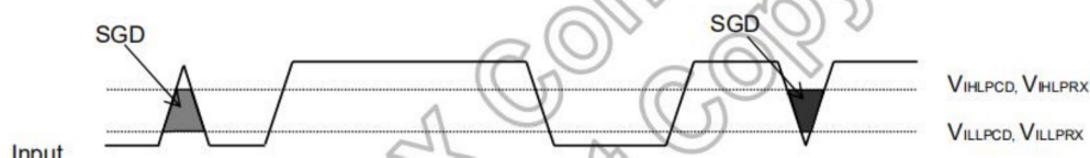
Input glitch rejections of low-power receivers
