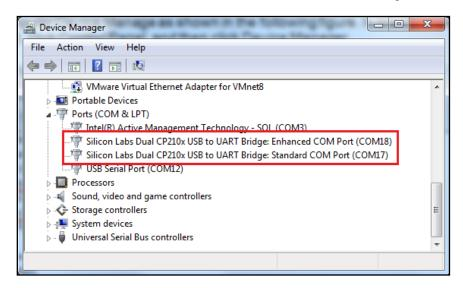
Open UART properties. Expand Ports (COM & LPT), right-click on Silicon Labs Dual CP210x USB to UART Bridge: Enhanced COM Port (COM17), and then click Properties. CPM17 will be connected to the PS UART0 and COM18 will be connected to the PS UART1. In this tutorial, we will be using the PS UART0 as STDOUT and STDIN.
