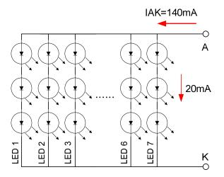
Note(6) When LCM is operated over  $60^{\circ}$ C ambient temperature, the IAK of the LED backlight should be adjusted to 105mA max
