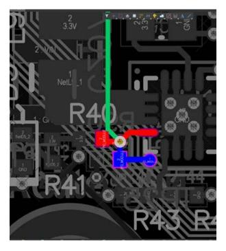
Figure 12 – PG\_MODULE location on MicroZed
