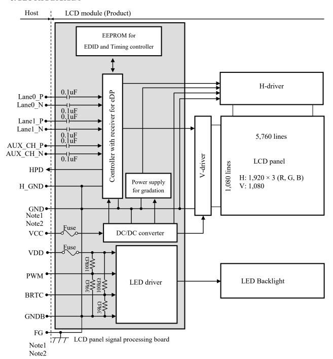
Note1: Relations between H\_GND (High Speed Ground), GND (Signal ground), GNDB (LED driver ground) and FG (Frame ground) in the LCD module are as follows.
