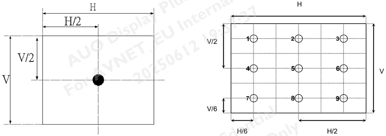
5. Viewing angle is the angle at which the contrast ratio is greater than 10. The angles are determined for the horizontal or x axis and the vertical or y axis with respect to the z axis which is normal to the LCD surface. For more information see FIG3.
