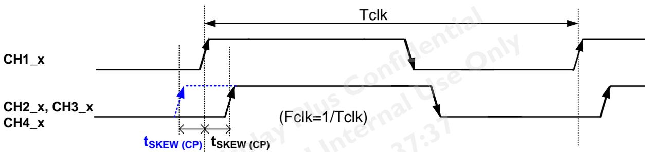
Note3. LVDS Receiver Clock SSCG (Spread spectrum clock generator) is defined as below figures.
