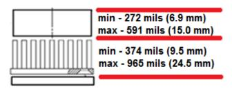
Figure 30 – UltraZed-EV SOM Fan and Heatsink MIN/MAX Combinations
