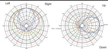
NOTES: Frequency response measured at 4m (13.12ft). For better detail, only light smoothing (1/12th octave) has been used. Polars were acquired by placing the unit on a computer controlled turntable inside a 300 m³ (10594 ft³) anechoic chamber. Measurement distance is 4m (13.12ft).
