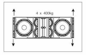
The maximum number of units that can be suspended from the AX-AERO50 flying grid is 16. The maximum limits established by the manufacturer should never be exceeded.
