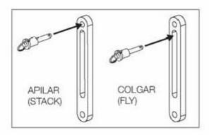
All of the elements needed to rig or stack the systems are integral to the enclosure (G1A50, G2A48 and the quick release safety pins). The additional items needed are the AX-AERO50 rigging structure (bumper bar), chains and hoists, the PL-50 dolly platforms and the AX-COMBO12 rigging adapter.
