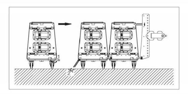
Proceed to attach the remaining units in the same manner until all the array units are attached to one another. For example, if we are assembling a six unit array, the process will be repeated six times. When all the units are attached, the complete array is ready to be hoisted.
