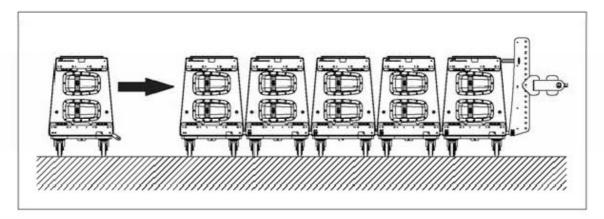
The complete assembly should begin being lifted from the hoist (3) so that the rear of the enclosures come together due to their trapezoidal shape. The hoist will be used only to take up slack in the chain, all the weight should be on the hoist. Proceed in this manner until the wheels of the last enclosure are off the ground. From here on, the array can now be lifted with the hoist.
