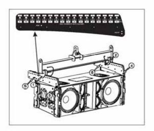
Once the first box is attached to the structure, the remaining boxes should be brought to the array and attached repeating the previous steps (1 and 2) using G1A50 guides and safety pins per side making sure that the pins have been inserted and locked correctly.
