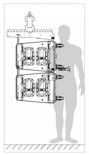
Once the boxes have been joined, the front dolly panels can be removed. The next boxes should be attached "one by one" using the methods described. Finally, the array should be hoisted to the correct height and secured with slings to avoid swinging.
