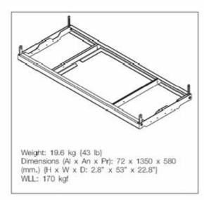
The AX-COMBO12 is joined to the last aero 50 cabinet using G1A50 and G2A48 included steel guides and 6 quick release pins. The angle depends on the hole of the rigging structures where the pins are inserted, through the slots of G2A48. The first aero 12A unit is joined to the AX-COMBO12 using its G1A and G2A included steel guides and quick release pins.
