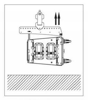
Once the first box has been placed at 0° and raised approximately 75cm (30 in) the second box of the array can be placed nearby. Once located in position, the G2A48 guides of the second box should be freed and inserted in the rear located receiving points of the suspended box and secured with the safety pins.
