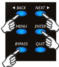
There are nine bands of parametric equalisation available on every output. The behaviour of each individual band can be changed to a variety of different filter shapes, including high and low shelves. Changing the filter type is achieved by pressing BYPASS to bypass the filter and then pressing ENTER during editing any particular band. For more details about the various types of filter available, please see page 27.
