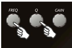
Note: The delay steps are 1mS (343mm) through FREQ, or 10uS (4mm) through Q encoder.
