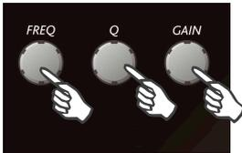
Using FREQ, the attack time change. Through Q the release time change, and through GAIN the threshold change. To complete the procedure, press ENTER.
