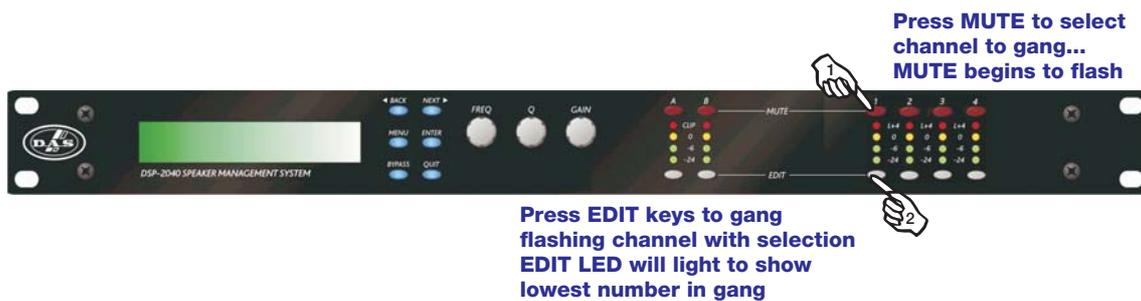
Press a MUTE key to choose the output to gang – its LED will begin to flash, and an EDIT key will illuminate to show which output it is currently ganged with. To change this selection, just press another EDIT key, remembering that gangs work from the highest to lowest number. So, to gang outputs 1 and 4, press MUTE 4 then EDIT 1 – the display will show
