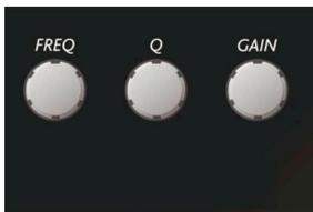
**[8]-Rotary Encoders:** Three velocity sensitive encoders adjust the relevant parameters as displayed on the screen.
