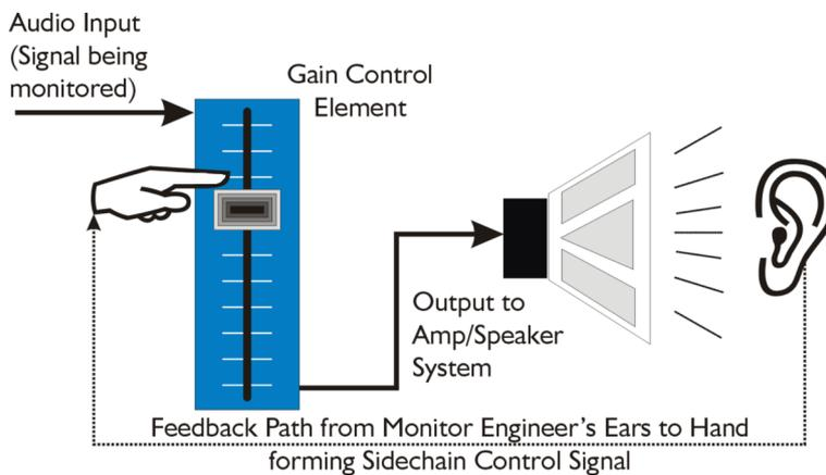
There is a hidden sidechain in operation even in this case. The main signal path is fed through the monitor desk and the gain controlled by adjusting the fader. The sidechain is formed by the feedback path between the engineer's ears checking the level and his brain instructing his hand to turn the fader down if the volume goes over the threshold he has chosen.
