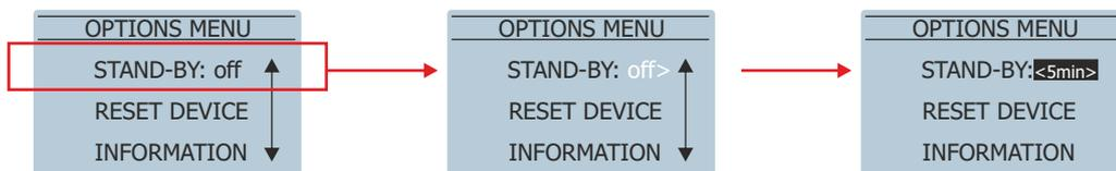
STAND-BY: When no signal is detected the amplifier shuts down. Time can be selected
