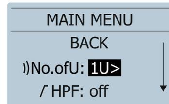
The available options for "No.ofU" are: 1, 2, 3, 4, 5 depending on the size of the array. Rotate the encoder to select the option needed and press again to confirm.
