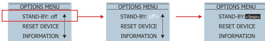
**STAND-BY:** When no signal is detected the amplifier shuts down. Time can be selected
