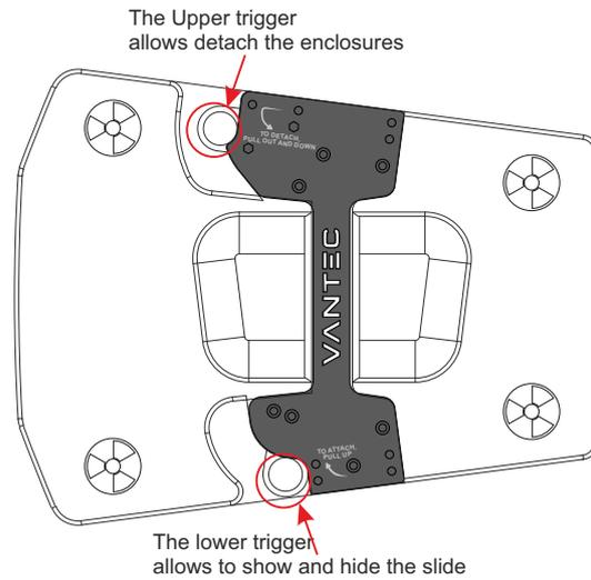
Moving the lower trigger up (1), reveals the slide that will fall by its own weight (2). When releasing the trigger, it will return to its place and the slide will remain fixed (3).
