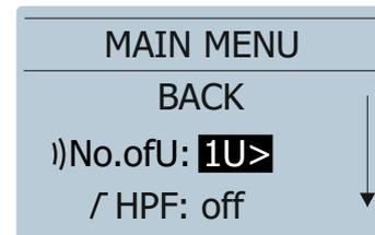
The available options for "No.ofU" are: 1, 2, 3, 4, 5 depending on the size of the array. Rotate the encoder to select the option needed and press again to confirm.
