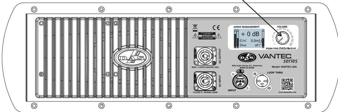
**Note:** The INPUT and LOOP THRU are type XLR balanced connectors.
