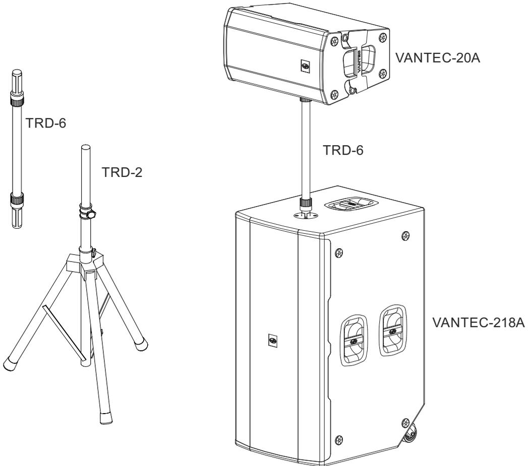
Example of VANTEC-20A on VANTEC-218A with TRD-6
