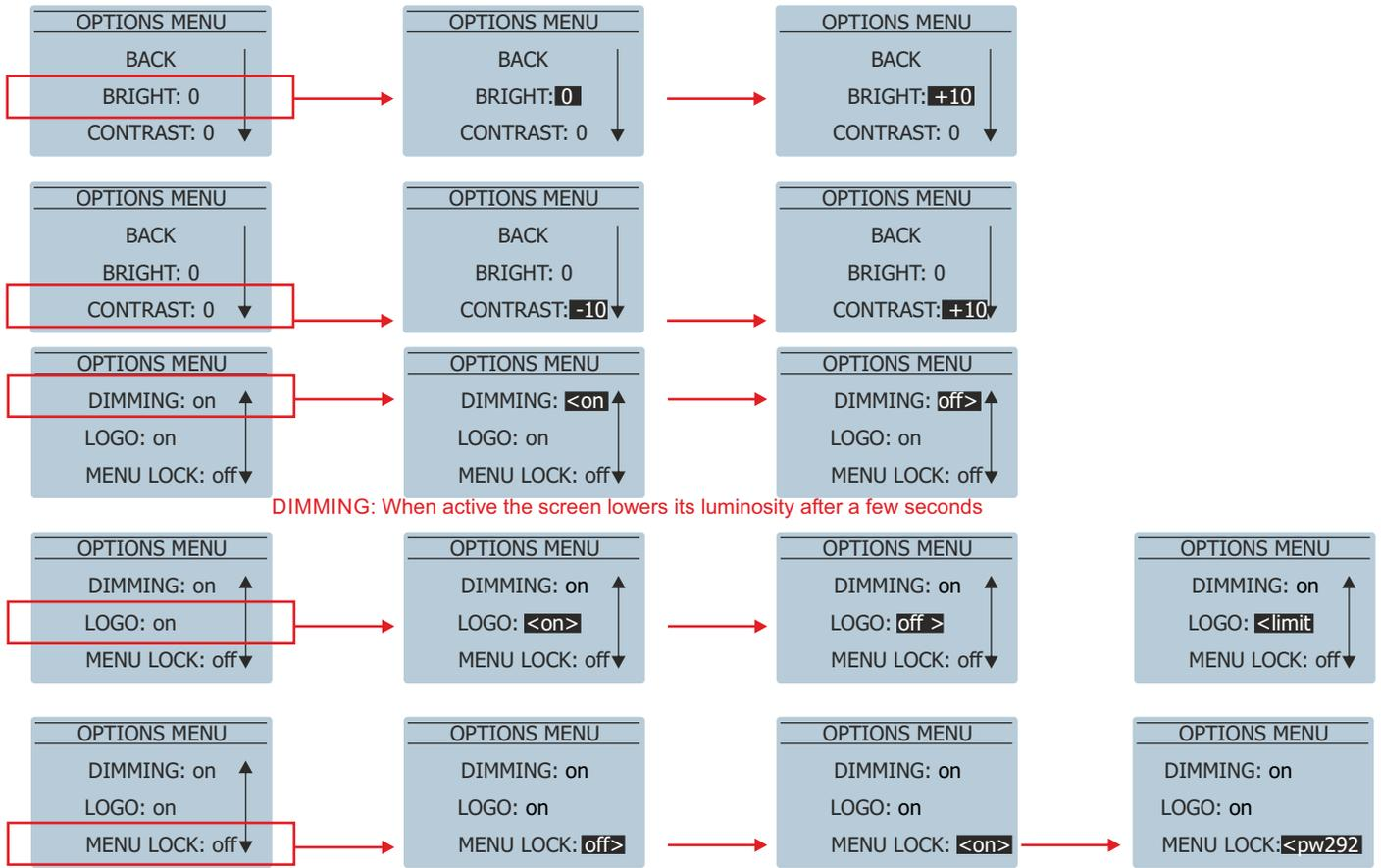
**DIMMING:** When active the screen lowers its luminosity after a few seconds
