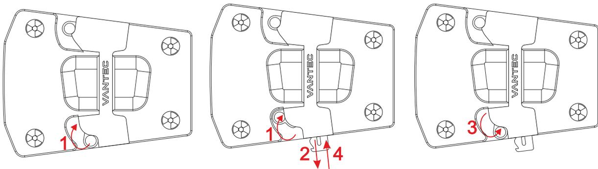
Similarly, to hide the slide we must act on the trigger as in (1) and push the slide up (4), releasing the trigger (3), finally.
