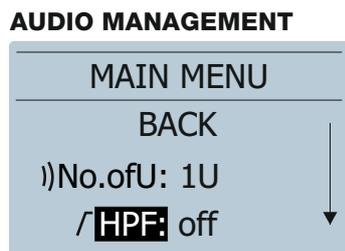
Rotate the encoder and press to confirm one of the following "HPF" options: off, 63Hz, V118A, 100Hz.
