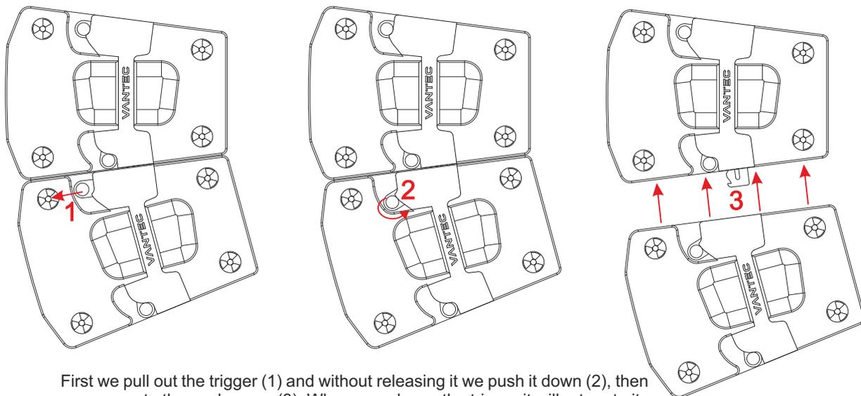
First we pull out the trigger (1) and without releasing it we push it down (2), then we can separate the enclosures (3). When we release the trigger it will return to its position. Finally, we would hide the slide as indicated on the previous page.
