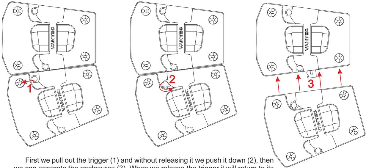
First we pull out the trigger (1) and without releasing it we push it down (2), then we can separate the enclosures (3). When we release the trigger it will return to its position. Finally, we would hide the slide as indicated on the previous page.
