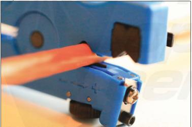
The CSR-1575 also includes a blade for the longitudinal cut. The reversible V-block should be positioned to accommodate a larger diameter cable. After setting the blade depth, position the blade at the beginning of the window, firmly close the tool and pull the tool towards the end of the window. A nice cut will be the result and the jacket can be easily removed.
