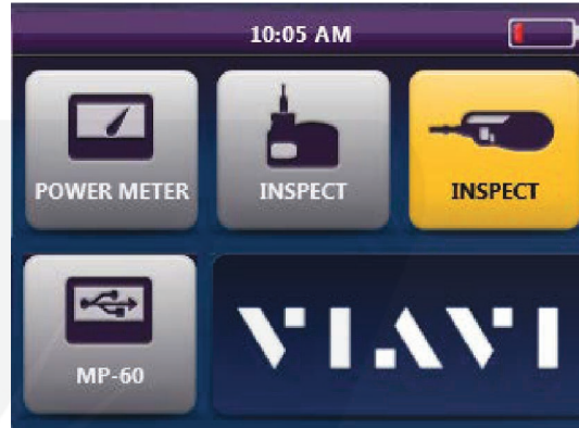
Fig. 1: OLP-82P Home Screen shown with P5000i Probe and MP-series USB OPM attached via USB
