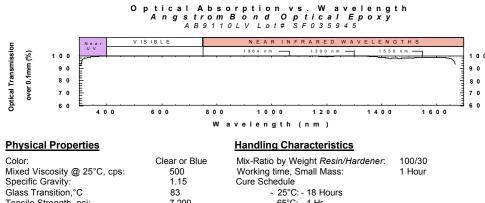
Tensile Strength, psi: 7,200 Hardness, Shore D: 79 Dielectric Strength, Volts/Mil: > 400 Coefficient of Thermal Expansions, 54 x 10<sup>-6</sup> cm/cm: Operating Temperature Range, °C: Index of Refraction: -270 to 125 1.564
