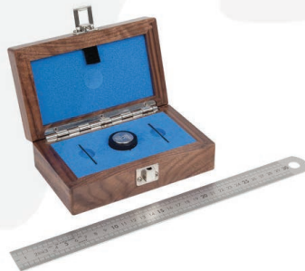
MPX Geometrical Calibration Artefact (Optional)
