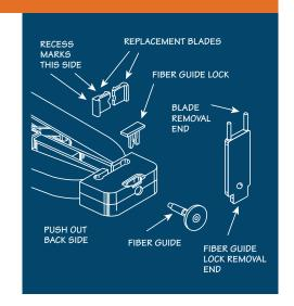
**Note:** Blades are color coded and matched to diameter and color of fiber guide lock. Replace or install fiber guide and fiber guide lock as needed. Always test strip fiber after installing new blade set. Remove blades periodically and clean with brush provided and alcohol.
