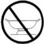
Do not place the pans directly on the burner.
