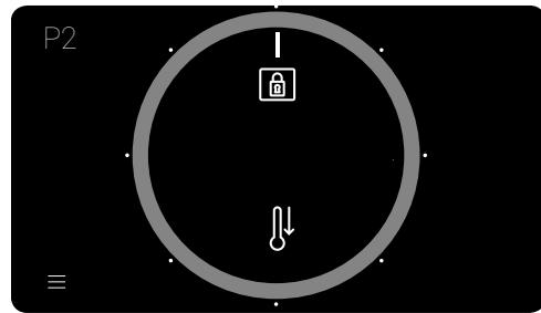
When the door is unlocked and can be opened, the symbol will disappear and the time will be shown again on the clock display.
