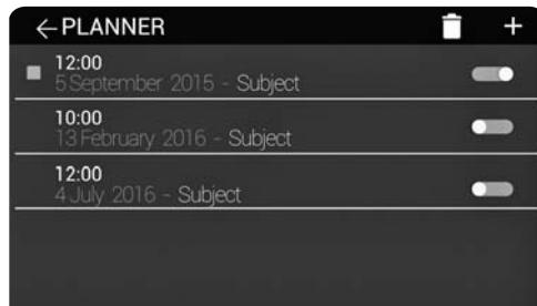
To add a new entry, press on the symbol . The screen for entering the date and time of the reminder is displayed. The buttons **Cancel** (to cancel the entry), **Next** (to enter a name for the entry) and **Finish** (to confirm the entry with
