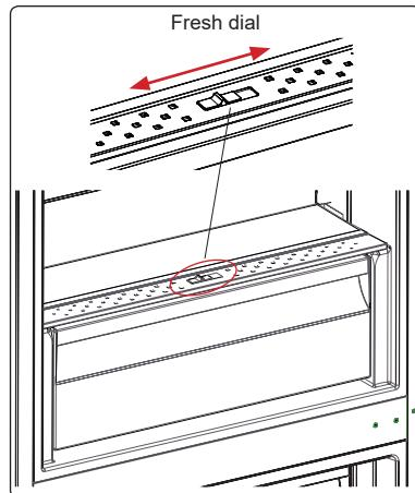
If the VitaCare Box is full, the fresh dial located in front of the crisper should be opened. This allows the air in the VitaCare Box and the humidity rate to be controlled, to increase the life of food within.
