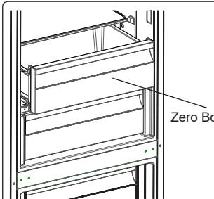
Keeping food in the Zero Box compartment, instead of the freezer or refrigerator compartments, allows food to retain freshness and flavour for longer, while preserving its fresh appearance. When the Zero Box tray becomes dirty, remove it and wash with water.
