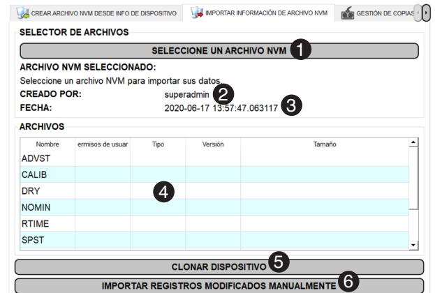
NVM files are imported to a unit to analyse the data collected in another unit in real time or to establish the parameters of the files in your unit and therefore "cloning" the original one.
