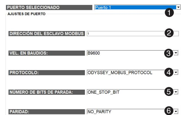
The communications window allows you to configure and change the parameters of the different communication ports available in the device.
