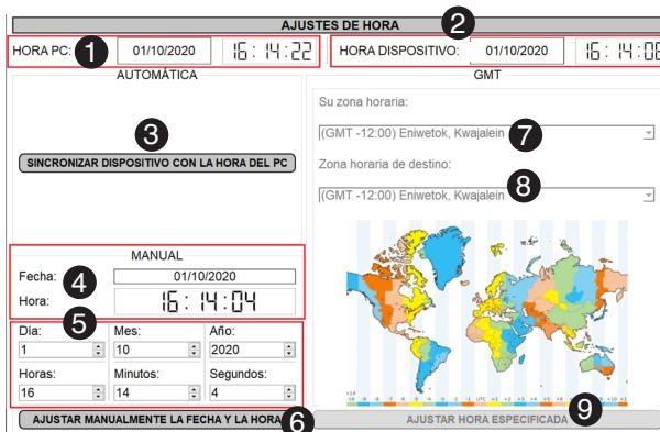
This device configuration window allows you to view the time of the device (2) and of the computer (1) and to configure its time using the explorer, either manually (6) or automatically (3).
