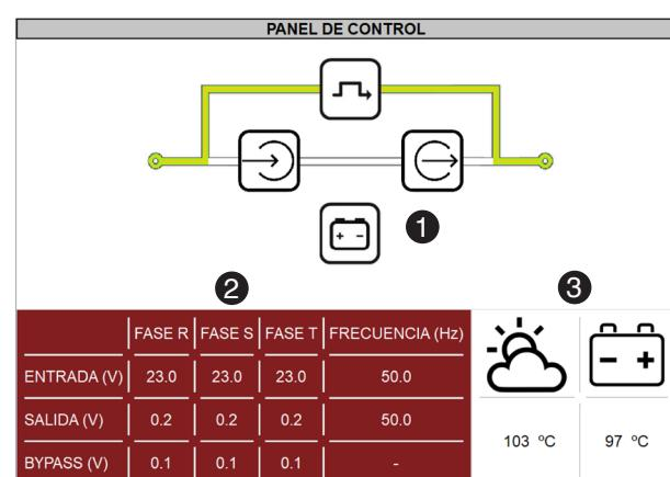
This window is to be used for interface landing, to find out the status of your ADAPT2 unit at a quick glance, giving you graphic view of the current flow in your device (1), temperature (3) and main voltages (2).
