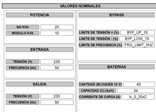
This window shows the key parameters that define the device, such as the input and output voltages and its power supply (kVA).
