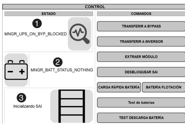
This window gives you general control of the UPS status using the commands located on the right; on the left we can observe some of the more generic status indicators of the device such as UPS status (1), battery status (2) or status of the modules as a whole (3).
