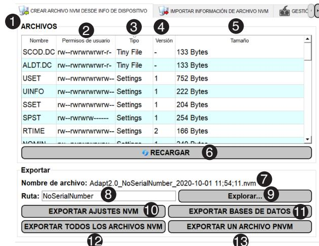
This section of the NVM file system allows you to extract the information stored in these NVM files in the form of a file for later use, processing or analysis.
