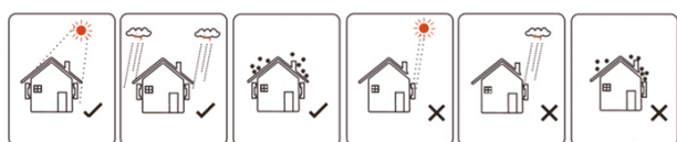
Fig. 17. Recommended locations for the inverter.
