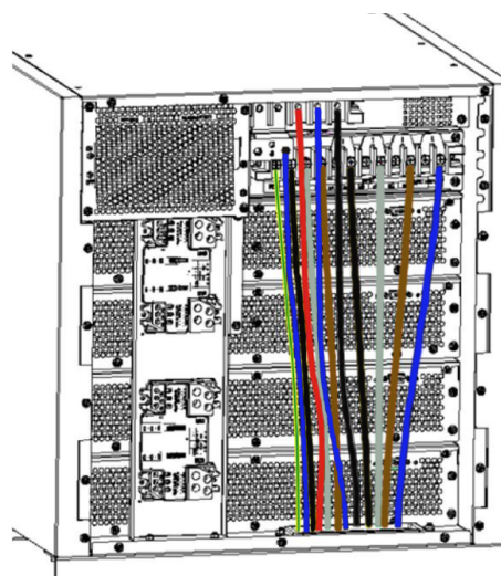
Cables entering through the base.
