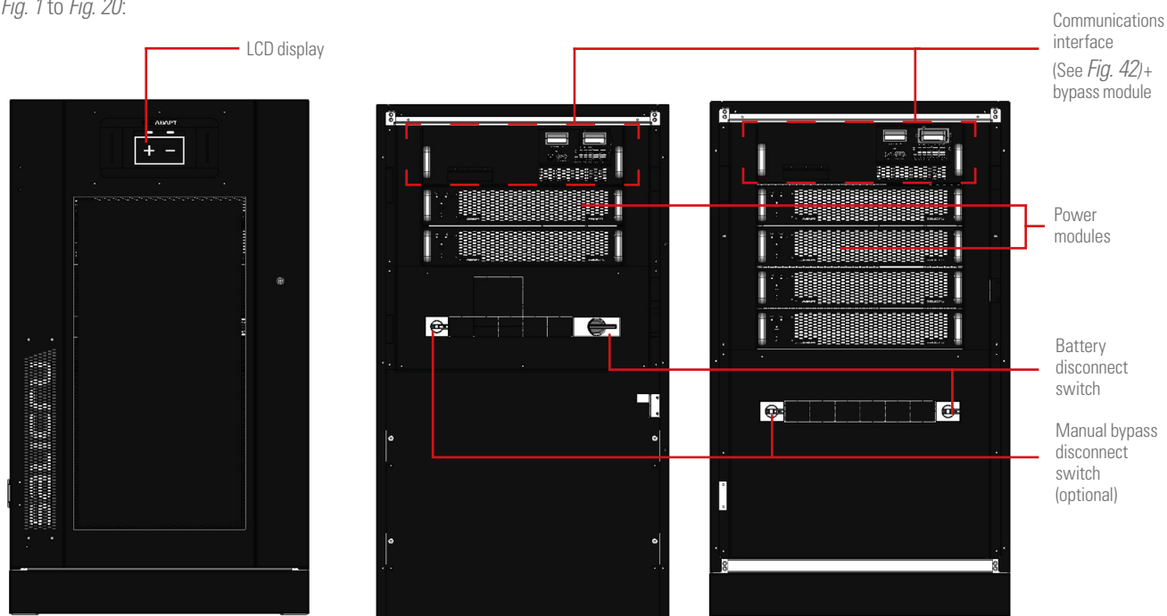
Fig. 1. Front views of the 24U cabinet, with the door closed (left) and the door open with 2 and 4 x 10 and 15 kVA modules installed (centre and right, respectively).
