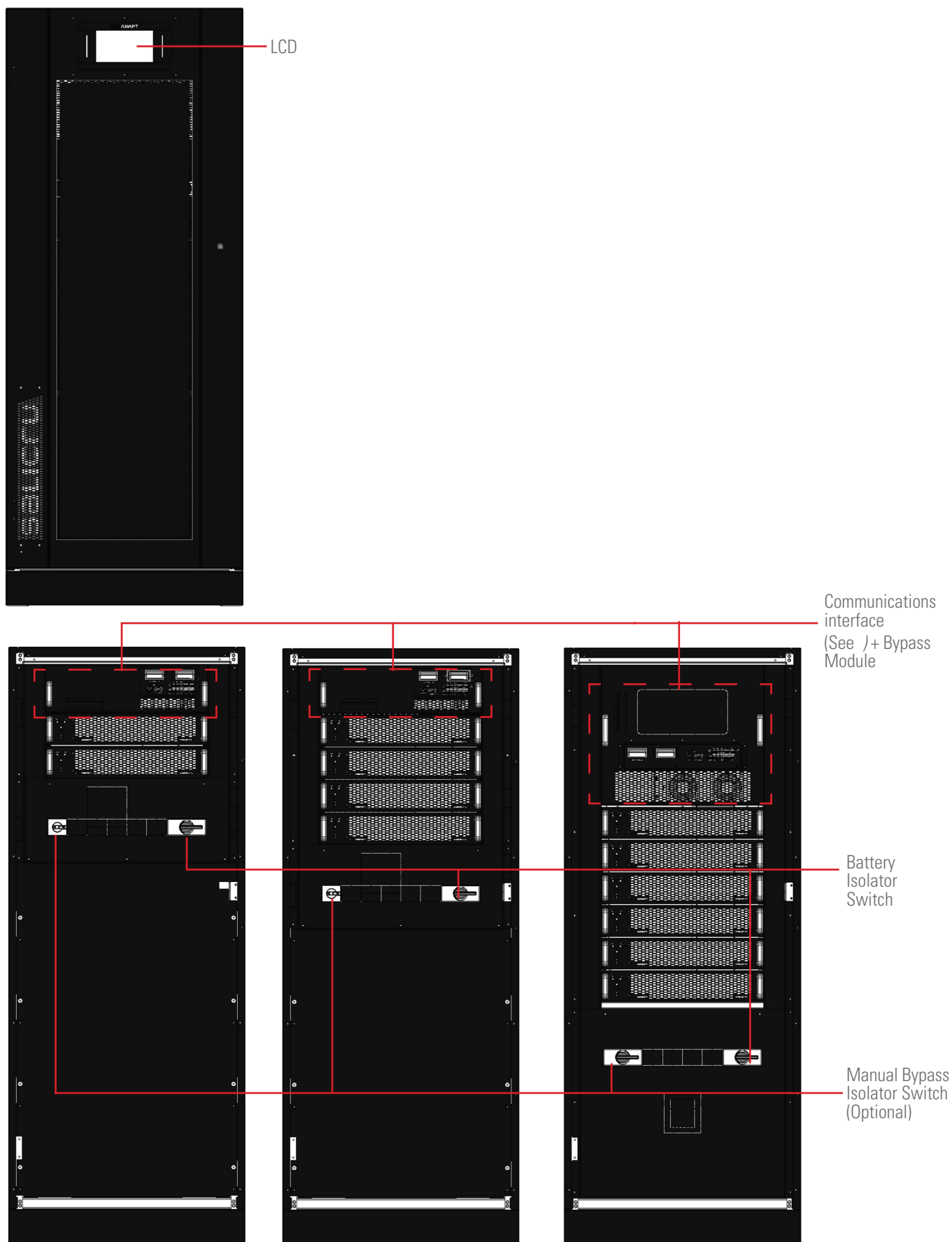
Fig. 3. Front views of the 33U cabinet, with the door closed (above left) and the door open with 2, 4 and 6 modules installed (below).
