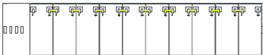
Fig. 28. Top view of a row of batteries (12 V, 7-9-11 Ah).
