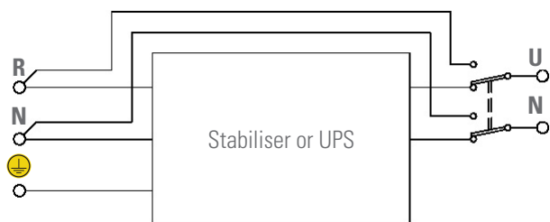
Fig. 2. Single phase / Single phase equipment's block diagram with Bypass type B1*.
