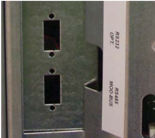
Picture 2 – Mounting position of the SLOT-REM-PV card (100...800kVA series FXS)
