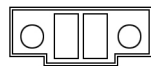
Fig. 23. Terminal block for connection to the inverter shutdown auxiliary contact of the manual bypass board.
