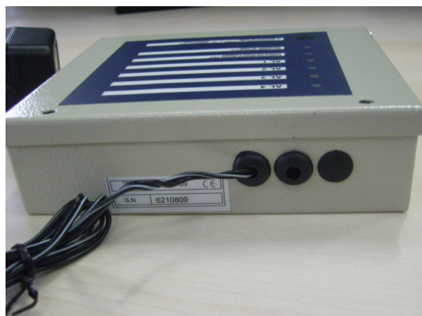
Fig. 18. Remote panel: cable hole
