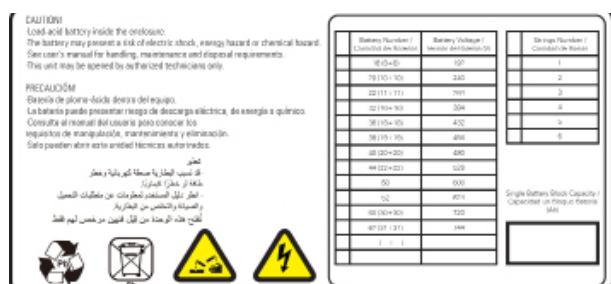
Fig. 40. Battery configuration label affixed to the equipment.
