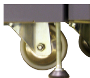
Element ( PB ) tighten against the floor.
