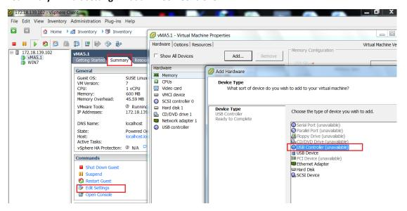
Choose the critical guest OS that Winpower is installed, Add the USB device by the "Summary"->"Edit setting"->"add"->"USB device", make sure the UPS is connected.
