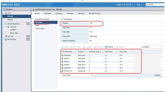
Please don't check the box "Shutdown all the VMs before host shutdown", so Winpower only shut down the hosts. The VMs will be shut down before host shutdown by the "Autostart" function.
