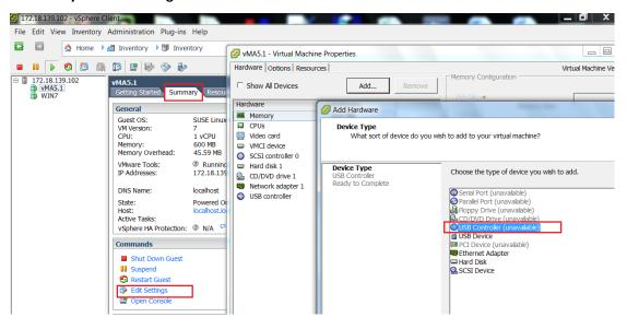
Choose the critical guest OS that Winpower is installed, Add the USB device by the "Summary"->"Edit setting"->"add"->"USB device", Choose "prolific USB-Serial Controller", make sure the UPS is connected.
