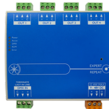
DMX/RDM Splitter - 1 channel input, 4 channels output A64791
