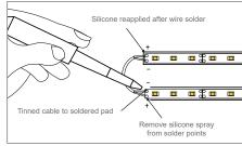
Please note drawings are an installation guide only. Each LED tape application may have variable factors. Cable size may need to be specified to limit the voltage drop throughout the circuit.
