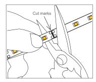
To provide a cable connection, cut and trim the cable to the appropriate length. Solder the wires onto the end of the LED tape ensuring the correct +/- polarity.
