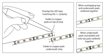
Please note drawings are an installation guide only. Each LED tape application may have variable factors. Cable size may need to be specified to limit the voltage drop throughout the circuit
