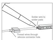
Cut and trim the wires to the appropriate length required. Thread wires through silcone connector power feed hole and solder wire to the soldering pads at the end of the LED ribbon strip. Ensure the correct +/- polarity to form a continuous electrical circuit.
