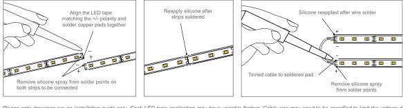
Please note drawings are an installation guide only. Each LED tape application may have variable factors. Cable size may need to be specified to limit the voltage drop throughout the circuit.
