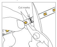
To provide a cable connection, cut and trim the cable to the appropriate length. Solder the wires onto the end of the LED tape ensuring the correct +/- polarity.
