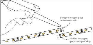
Please note drawings are an installation guide only. Each LED tape application may have variable factors. Cable size may need to be specified to limit the voltage drop throughout the circuit.
