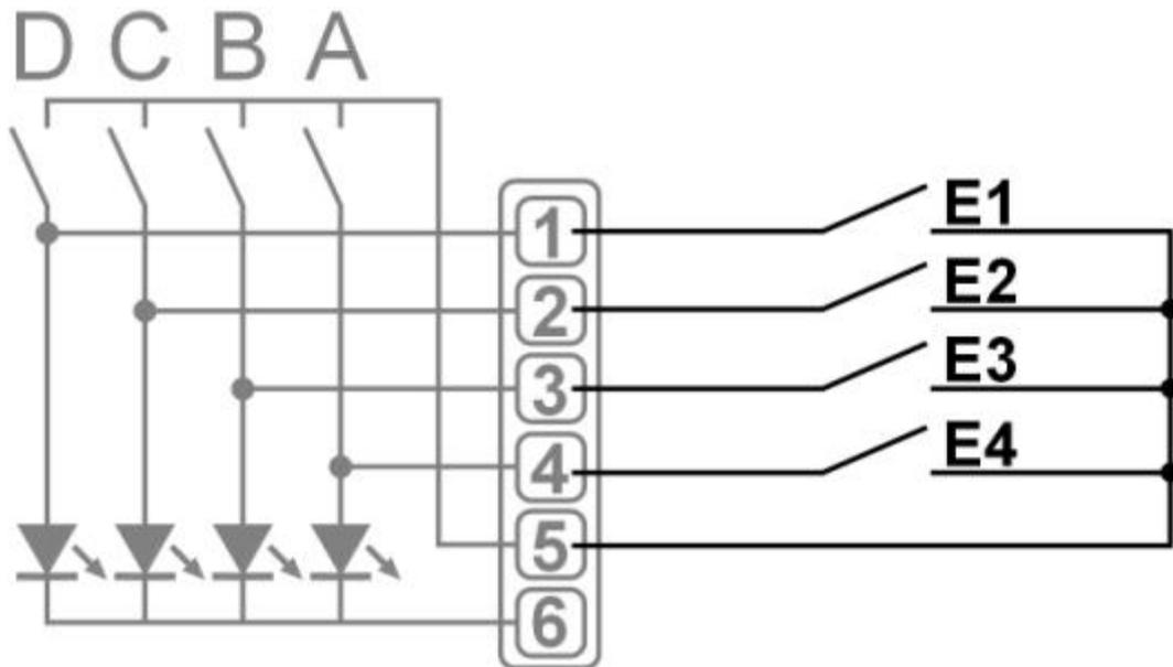
**Wiring diagram as Output with LEDs (Channels C and D) and Input (Channels A and B):**
