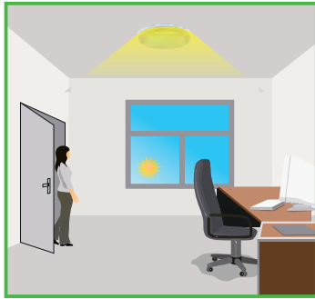
When the natural light is sufficient or dark, movement is detected and the light will turn on 100% brightness.
