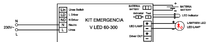
NO PERMANENTE/NON MAINTAINED
